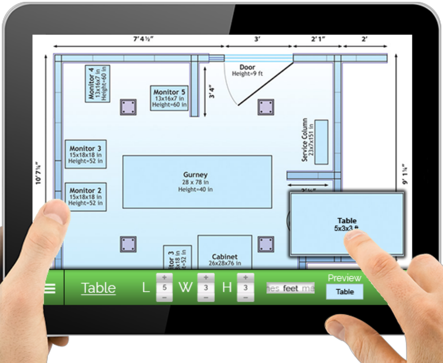
Figure 2. Map Generator (GUI) showing a sample building session. Objects are chosen with correct dimensions and dragged into place in accordance to the buildings structure to serve as 'detection zones' integrated with Third-Eye.
